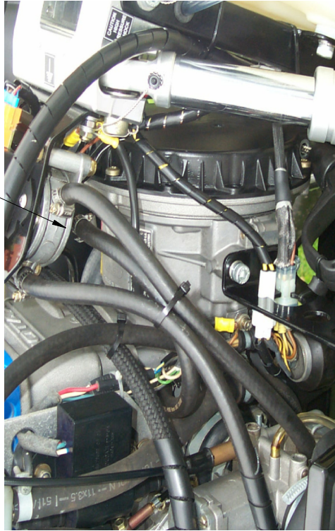
PHOTO 2. FUEL PUMP WITH HOSES
