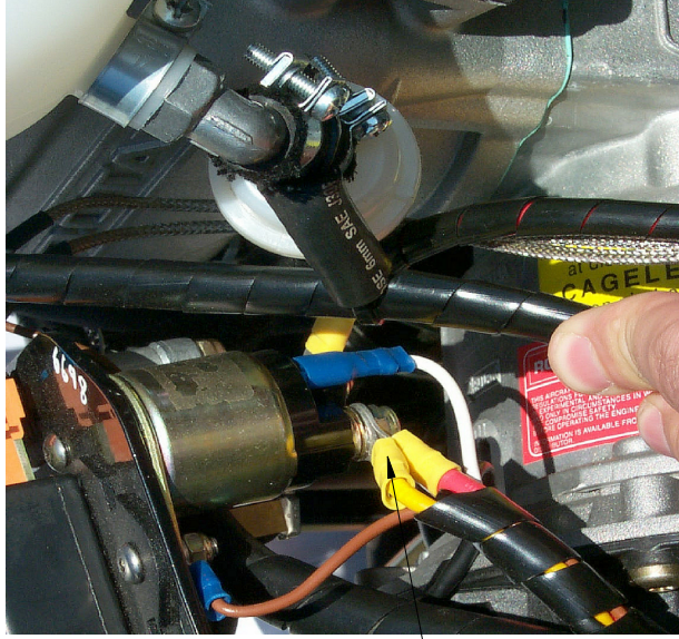
PHOTO SHOWS ATTACHMENT OF WIRES TO THE DATA BOX AND SOLENIOD.
