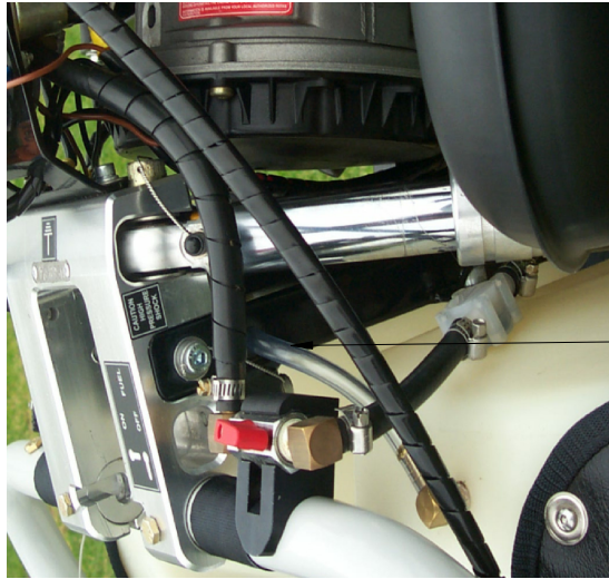
PHOTO 1. FUEL TAP WITH HOSES
