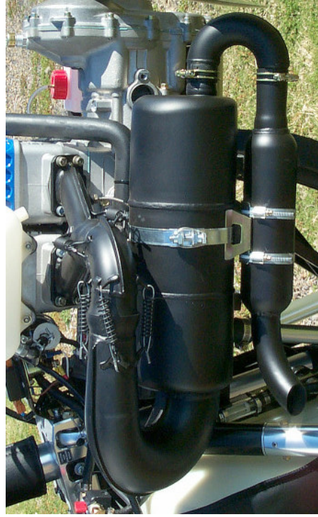
PHOTO OF INSTALLED EXHAUST WITH AFTER SILENCER.
