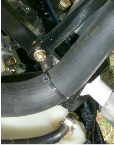
PHOTOS SHOW CABLE TIED FUEL HOSE SPACERS.
