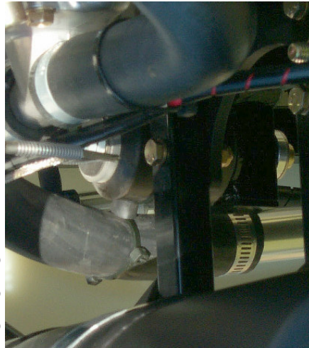
PHOTOS SHOW CABLE TIED FUEL HOSE SPACERS.
